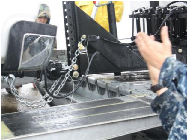
Figure 4: Tongue nearly touches ramp
