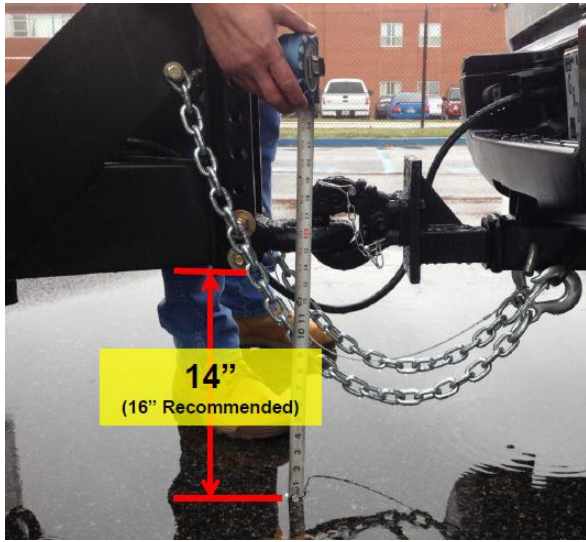
Figure 2: Distance from the ground to the bottom of the trailer frame. Should be 16" but was set to 14" for the validation load.
