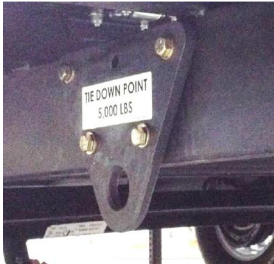
Figure 7: Tiedown Point (5K Rated Capacity)
