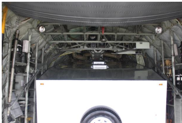
Figure 6: Trailer nearly touches C-130 Ceiling
