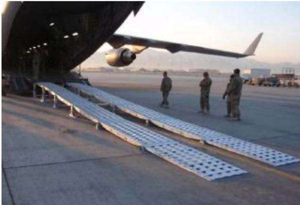
**Figure 6: Under C-17 Ramp Toes (in accordance with para 1.d.)**
