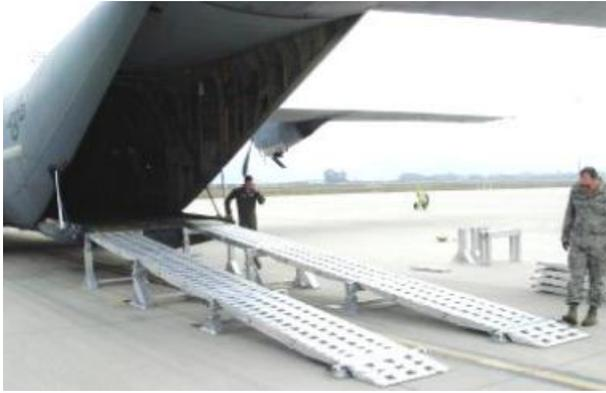
**Figure 4: C-130 Using Auxiliary Truck Loading Ramps**
