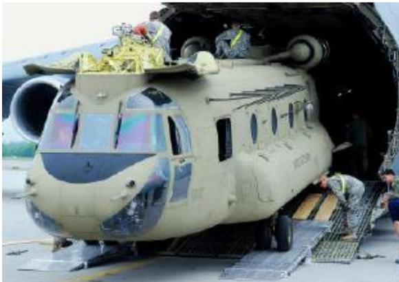
**Figure 8: CH-47 using Pooched Plate (in accordance with para 1.a.)**
