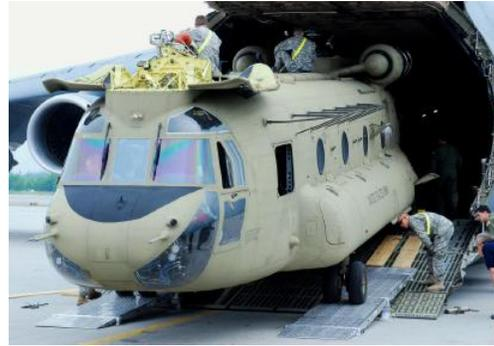
Figure 7: CH-47 using Poached Plate
