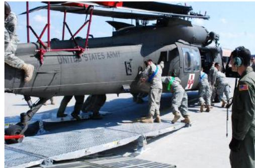
Figure 9: Loading UH-60 using Poached Plate Ramps
