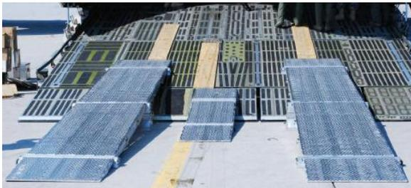
Figure 8: Combined 26K and 10K for loading UH-60 on a C-5
